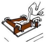
**Step 8:** After 20 minutes, take casting boards apart, scrape off top of plaster and bevel the edges slightly. Grasp opposite sides of the plaster/clay mold and gently twist to loosen clay from the work board as shown. Turn mold over and proceed to lift off clay from model and plaster half of the mold.
