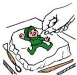
**Step 3:** When clay is all in place, smooth and leather hard, square off clay as shown. Using a soft brush, apply two thin coats of Orange Shellac over the object and the top surface of the clay parting line. After 15-20 minutes, apply talcum powder, dusting lightly.
