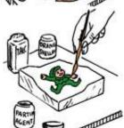
Step 5: Prepare your casting boards, wiping each with Parting Agent on front surface and edges. Assemble as shown with "C" Clamps. With wooden tool, seal edges where clay parting line meets the insides of the board as shown.
