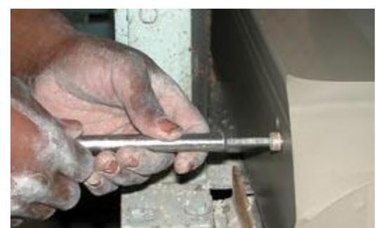
The “firmness” of every batch of clay is measured with a penetrometer.
